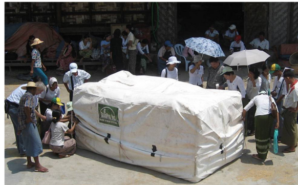
Hermetic Storage Cocoons control moisture and insects without pesticides, maintain milling quality, germination of seeds and protect grain from rodents, presented by Mr. Martin Gummert, Senior Scientist, Post Harvest Development International Rice Research Institute, Philippines
